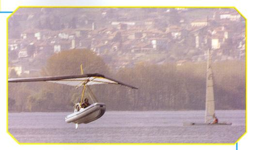
gets inside the boat deck. The standard wing is the well known La Mouette, Golf 19 (18.5 square meters). The Golf 19 was chosen after many tests because of its precision and the materials used. Tri-lam is a special fiber cloth used on Racing Sailboats, which can last up to 3 times longer in the UV rays, than Dacron or Mylar.
